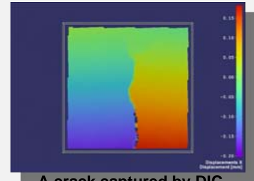
A crack captured by DIC
