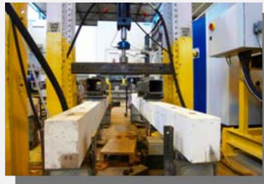
Cyclic loading experiments
