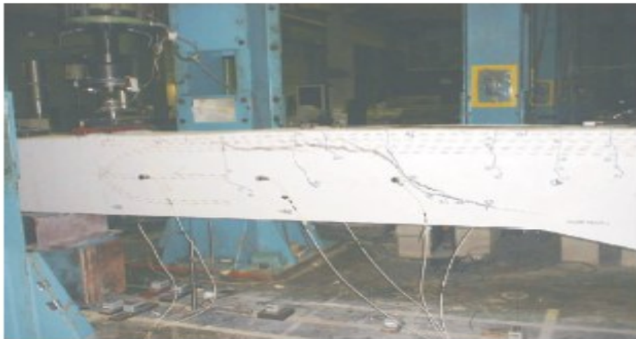
Figure 6.24: Beam HB2. Shear Failure.
