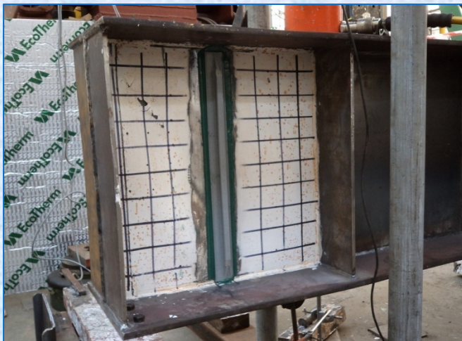
GFRP-strengthened Specimen (FL = 277 kN)
