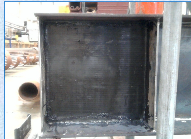
Carbon Fabric-strengthened Specimen (FL = 287 kN)
