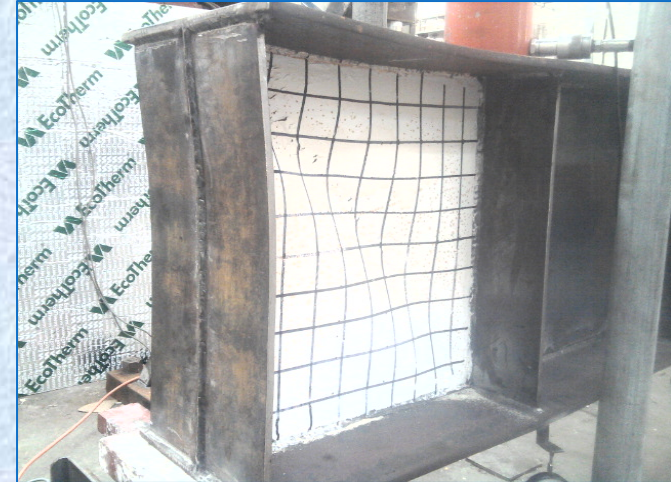
Control Specimen (Failure Load, FL= 230 kN)
